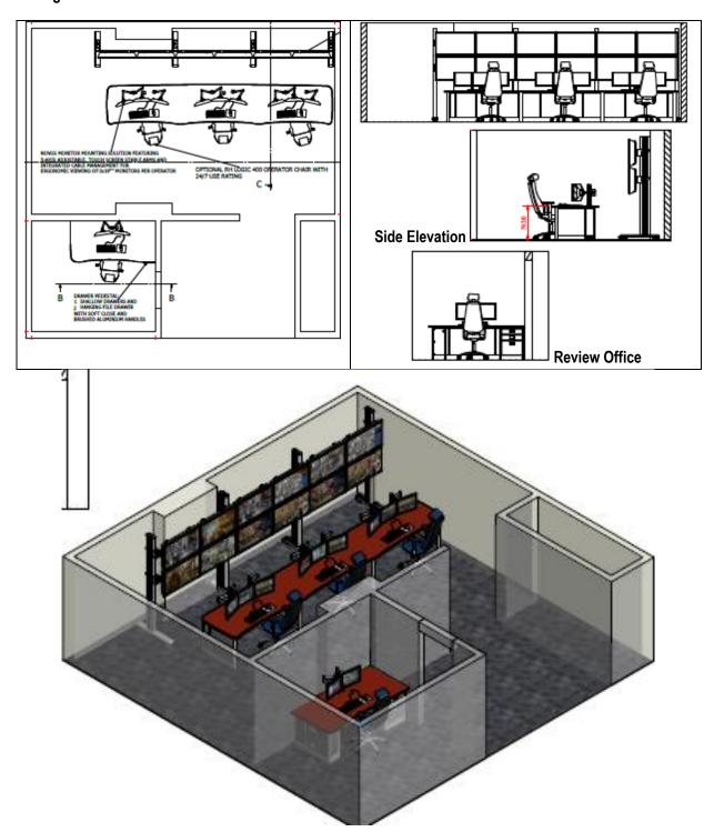
This design takes advantage of the current supervisor's office as a review office. Initial discussion with local management about re-utilising this office in this way made it clear that it would not have a negative operational effect. The whole flow of the room means that, although there are 3 workstations, they can operate across the same plane and at lease provide the opportunity for all 3 operators to work together.
