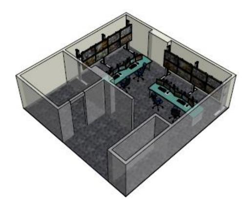
In addition to this a view of the actual layout in isographic format shows just how disjointed it would be. The supervisor's office couldn't effectively work as such without having a suitable window overseeing the room, but this wouldn't be feasible given the utility cupboard located in front of it. All in all this design did not provide the sort pf working environment conducive to an effective control room.
